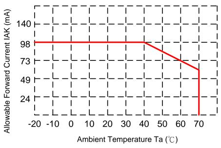
Note7 : This is panel surface temperature, not ambient temperature. Note8 : When LCM be operated over than  $40^{\circ}$ C, the life time of the LED back-light will be reduced.
